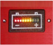
Turning ON the power the Trucharge indicator/diagnostic display will test the entire system for any faults before allowing the user to operate. This takes only 1 second and is usually done by the time the operator has put finger on the throttle. If display flashes, see "troubleshooting" below.
