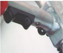
For powered operation of the system push finger throttle in the direction you wish to move. The throttle is true variable speed and will speed-up or slow-down according to how much pressure is applied.
