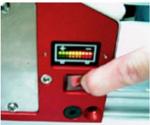
For safety reasons and to prolong the life of your battery, internal controller will automatically turn power OFF after 30 minutes of none-use.
