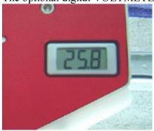
The digital voltmeter reads DC voltage from 14volts to 40volts. A typical charge will be at maximum capacity around 27.6volts.
