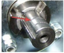
OUTER GROOVE ON TRANSAXLE SHAFT IN DISENGAGED (or unlocked)
