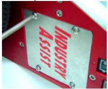
The screws are held in place with retaining clips making sure they are not lost.
